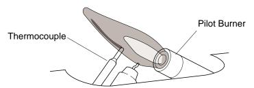
Figure 18 - Correct Pilot Flame Pattern
